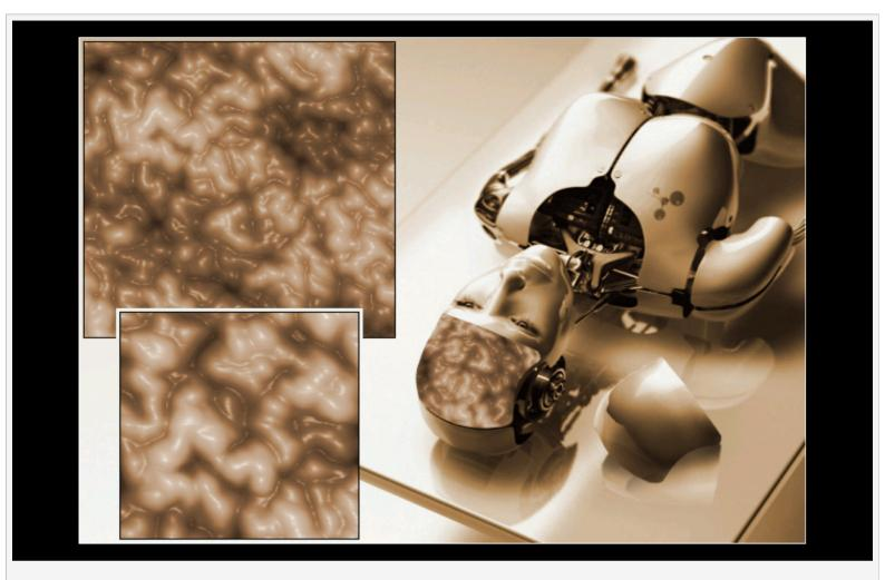
A surface resembling the gyri of a human brain is obtained after deposing a nanometer thick carbon film on a polyurethane substrate. The carbon film deposition is carried out by using the technique of pulsed arc plasma sputtering of a graphite target. During the deposition, the carbon film gets shrinked causing a deformation of the smooth surface of the polymer. As a result of the deformation, "nanogyri" are formed that have 73 nanometers in mean width and 13 nanometers in mean height.
